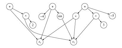
$$\begin{array}{l} \min x_1 + x_2^2 \\ \text{s.t.} \ x_1 + \sin x_2 \le 4, \ x_1 x_2 + x_2^3 \le 5 \\ x_1 \in [-4, 4] \cap \mathbb{Z}, x_2 \in [0, 10] \cap \mathbb{Z}. \end{array}$$
